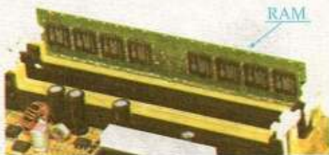
Fig. 1.1.3a RAM is plugged in a socket
