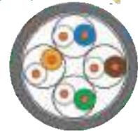
Figure 1.10 Twisted Pairs Cables
