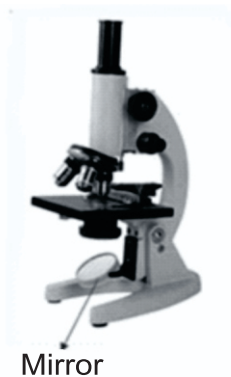
Figure 10.14: Mirror is used for the reflection of light into the microscope.
