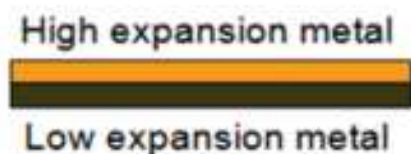
Fig. 9.10 Bimetallic Strip
