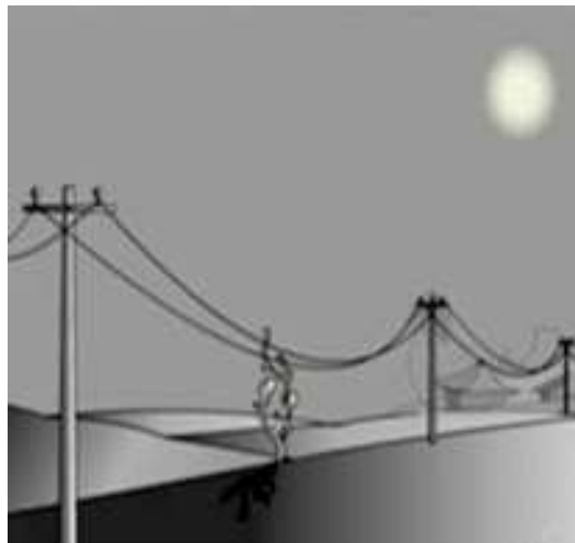
Fig 9.4 Electrical Wires are left slack
